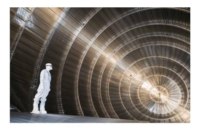
Photograph of the electron spectrometer used by KATRIN. Credit: KATRIN
