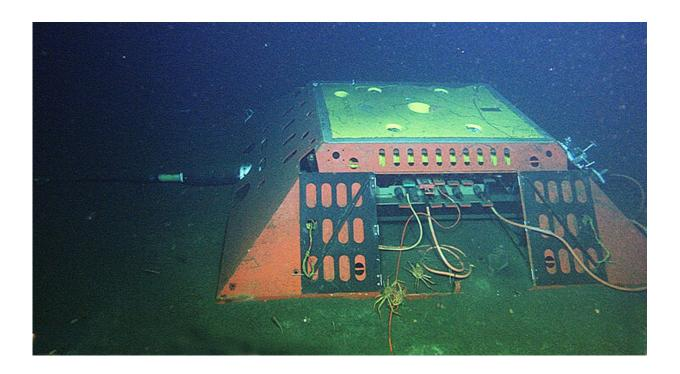
The Monterey Accelerated Research System (MARS) cabled observatory, a node for science instruments on the ocean floor 891 meters (2,923 feet) below the surface of Monterey Bay, is connected to shore by a 52-kilometer (32-mile) undersea cable that carries data and power. About 20 kilometers of the cable was used to test a new concept called photonic seismology on the seafloor. Credit: MBARI, 2009
