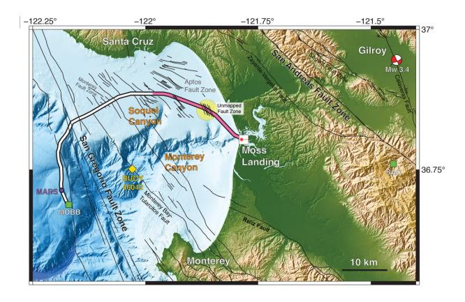
Researchers employed 20 kilometers (pink) of a 51-kilometer undersea fiber-optic cable, normally used to communicate with an off-shore science node (MARS, Monterey Accelerated Research System), as a seismic array to study the fault zones under Monterey Bay. During the four-day test, the scientists detected a magnitude 3.5 earthquake 45 kilometers away in Gilroy, and mapped previously uncharted fault zones (yellow circle). Credit: Nate Lindsey, UC Berkeley
