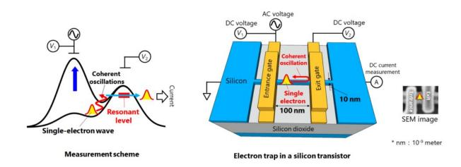
KAIST researchers have reported the detection of a picosecond electron motion in a silicon transistor. This study has presented a new protocol for measuring ultrafast electronic dynamics in an effective time-resolved fashion of picosecond resolution. The detection was made in collaboration with Nippon Telegraph and Telephone Corp. (NTT) in Japan and National Physical Laboratory (NPL) in the UK and is the first report to the best of our knowledge.
