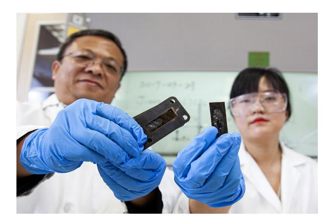
Professor Zhiyong (Richard) Liang and research faculty member Ayou Hao holding pieces of carbon fiber reinforced polymer composites with a protective heat shield made of a carbon nanotube sheet that was heated to a temperature of 1,900 degrees Celsius. Credit: Florida State University
