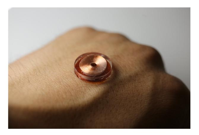
The 32 actuators—each the size of a small coin—vibrates to create the perception of touch
