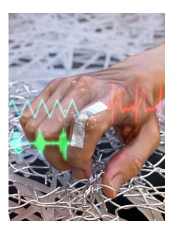
A photo of the film attached to a person's finger. It can be used as a wearable sensor to monitor heart rate and other movement. Reproduced, with permission, from Ref. 1 © 2019 Wiley-VCH Verlag GmbH & Co. KGaA, Weinheim
