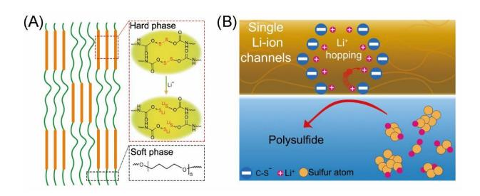
(A) Schematic diagrams of the formation of the polymer with the single-ion channels. (B) Schematic diagrams of single-ion channels regulate the polysulfide and Li-ion hopping. Credit: ©Science China Press
