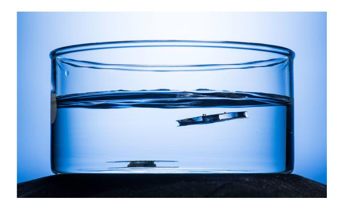
A metallic structure etched lasers, right, floats to the top on the water's surface in professor Chunlei Guo's lab. Credit: University of Rochester photo / J. Adam Fenster
