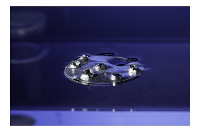
The superhydrophobic structure remains afloat even after significant structural damage -- punctured with six 3-mm diameter holes and one 6-mm hole. Credit: J. Adam Fenster/University of Rochester
