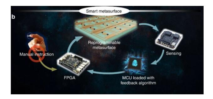
The schematic of a smart metasurface and the proposed method of study. The closed-loop system of the smart metasurface, which includes a digital-coding metasurface, an FPGA, a sensor, and a microcontroller unit (MCU) loaded with the fast feedback algorithm. Credit: Light: Science & Applications, doi: 10.1038/s41377-019-0205-3
