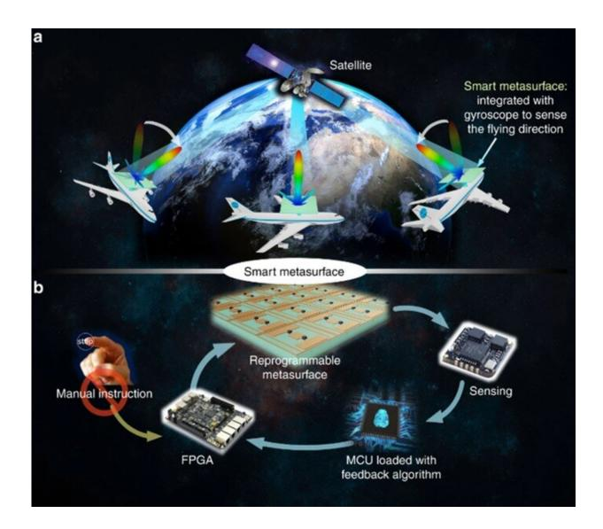
The schematic of a smart metasurface. (a) Illustration of the proposed smart metasurface with the self-adaptively reprogrammable functions without manual instruction. (b) The closed-loop system of the smart metasurface, which includes
