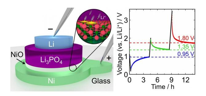
The stacked layers in the proposed memory device form a mini-battery that can be quickly and efficiently switched between three different voltage states (0.95 V, 1.35 V, and 1.80 V). Credit: ACS Applied Materials and Interfaces
