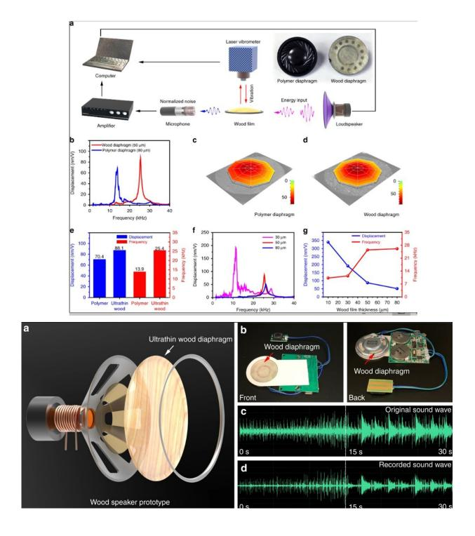
TOP: Acoustic properties of wood films. (a) Schematic of the vibrational frequency response measurement system. Insets: photographs of the commercial polymer diaphragm and ultrathin wood film. (b) The vibrational frequency response characteristics of the ultrathin wood film (50  $\mu$ m) and the commercial polymer (80  $\mu$ m) diaphragms. (c, d) The (0, 1) mode shapes of the polymer (80
