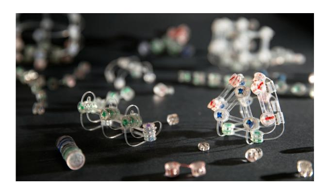
Acrylic panels containing tiny magnets were glued onto flexible mylar strips, forming the basic building blocks for researchers to explore the potential of magnetically controlled self-assembling systems. Credit: Lindsay France/Cornell University
