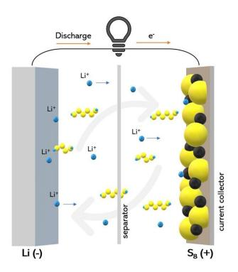
This diagram shows a lithium-sulfur battery during discharging. Scientists were able to observe how a certain type of electrolyte material can reduce the shuttling of polysulfide compounds (shown as yellow and blue chains) that impairs the battery's performance. Credit: Wikipedia/Creative Commons
