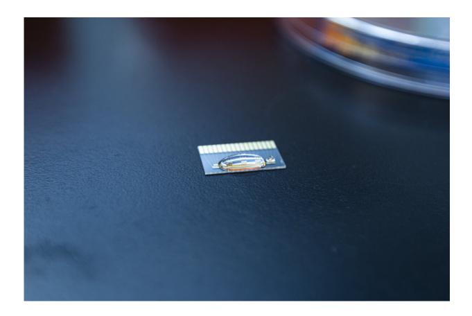
The new biohybrid system uses non-optical reporter enzymes contained within 16 microlitres of liquid which pair specifically with micropatterned electrodes hosted on a small chip no more than one inch in length. (To be visible, liquid shown here is more than 16 microlitres) Credit: Steve Southon
