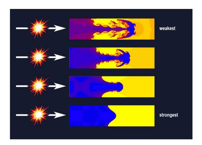
The application of stress to a solid causes the material to flow—a phenomenon known as Rayleigh-Taylor instability. This flow causes ripples patterned on the material surface to grow, forming jet-like structures coming off the surface. Credit: Shengtai Li and Hui Li/Los Alamos National Laboratory; adapted by APS/Joan Tycko
