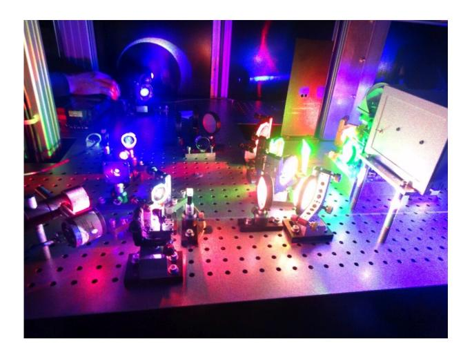
The new printer uses low-power continuous wave lasers to create holograms on a highly sensitive photomaterial developed by the researchers. Credit: C Yves GENTET
