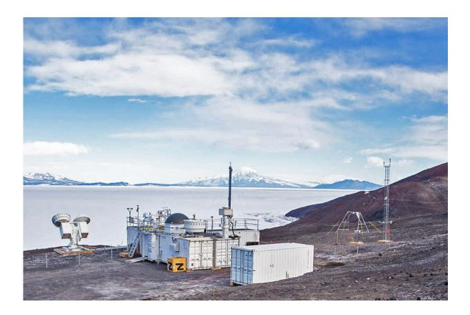
The Atmospheric Radiation Measurement (ARM) Mobile Facility (AMF2) was deployed to McMurdo Station, Antarctica, as part of a 14-month field campaign to gather sophisticated data with cloud radars and high spectral resolution lidar, and a complete aerosol suite. Credit: US Department of Energy Atmospheric Radiation Measurement (ARM) user facility
