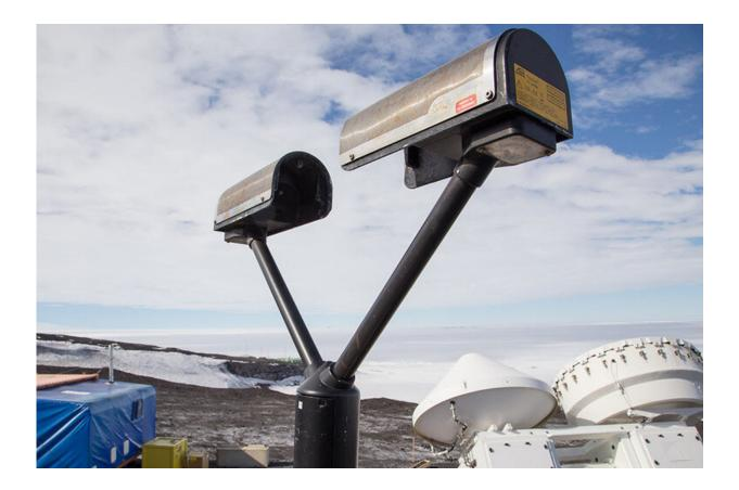
Sophisticated instruments, including laser disdrometers which measure precipitation as it passes through a fan-shaped laser-beam, collected data at McMurdo Station as part of the ARM West Antarctic Radiation Experiment (AWARE), a joint effort between the US Department of Energy and the National Science Foundation. Credit: U.S. Department of Energy Atmospheric Radiation Measurement (ARM) user facility
