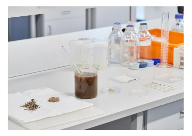
Banana pseudostem is dried, then powdered, then placed in alkaline solution to extract the cellulose, which is then processed into films of varying thicknesses. Credit: University of New South Wales
