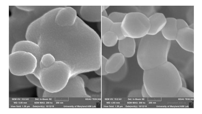
A team of Goddard technologists are experimenting with coated pigments to solve one of NASA's thorniest challenges: how to keep the orb's irregularly shaped, razor-sharp dust grains from adhering to virtually everything they touch, including astronauts' spacesuits. The uncoated pigment on the left looks smooth, while the coated pigment includes distinct features. Credit: NASA
