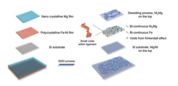
A schematic showing thin-film SSID for the Fe-Ni/Mg system. The thin films of Mg and Fe-Ni are layered on top of an Si substrate. Upon exposure to heat, the Mg dealloys Fe-Ni to form an Mg-Ni composite and pure Fe with a 3-D bicontinuous structure. Credit: *Materials Horizons*
