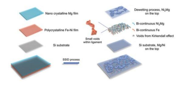
A schematic showing thin-film SSID for the Fe-Ni/Mg system. The thin films of Mg and Fe-Ni are layered on top of an Si substrate. Upon exposure to heat, the Mg dealloys Fe-Ni to form an Mg-Ni composite and pure Fe with a 3-D bicontinuous structure. Credit: *Materials Horizons*
