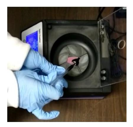
Drexel University researchers have developed a simple spin-coating method for making photo detectors, from a type of material called MXene, that could allow production to keep up with the demand for the devices in massive data centers and IoT technologies. Credit: Drexel University
