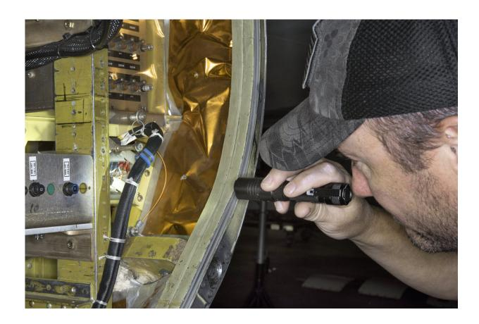
Ground crewman at NASA's Armstrong Flight Research Center in Palmdale, CA install a rail to support the Autonomous, Robotic Telescope Mount Instrument Subsystem, which is part of air-LUSI and has a camera that scans the sky to find the Moon. Credit: NASA Photo / Ken Ulbrich
