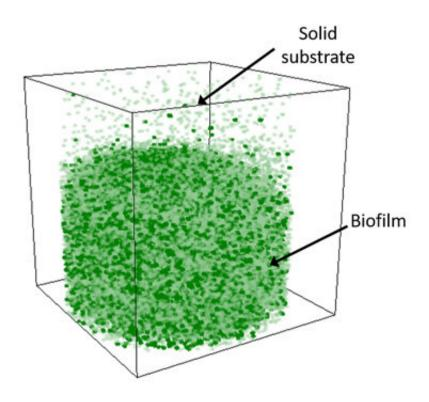
A 3-D molecular ion image allows scientists to track a PO<sub>3</sub> species in a live biofilm growing below a solid substrate. Credit: Environmental Molecular Sciences Laboratory
