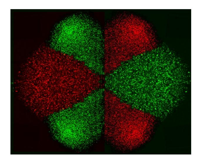
A dynamic pattern of different cell types isolated and deposited using the developed Micro-electro-fluidic Probe (MeFP). Credit: NYU Abu Dhabi faculty Mohammad Qasaimeh
