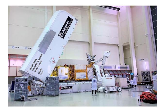
MetOp-SG's STM was transported to the ESTEC Test Centre in a protective, airconditioned container. Credit: ESA
