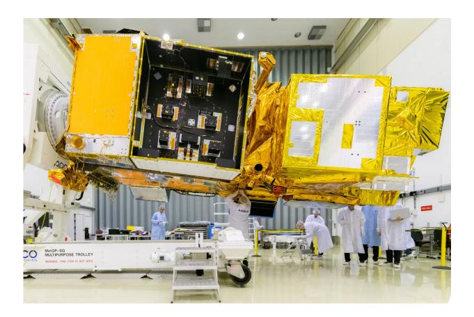
MetOp Second Generation's structural and thermal model during testing at ESA's ESTEC Test Centre in the Netherlands during summer 2019. Credit: ESA-SJM Photography
