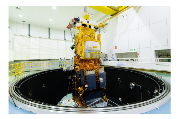
MetOp-SG's structural and themal model being lowered into ESA's Large Space Simulator, the largest vacuum chamber in Europe, ahead of thermal vacuum testing during summer 2019. Credit: ESA-SJM Photography
