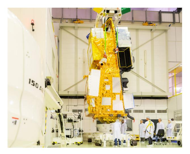
For MetOp Second Generation testing a prototype version specially built, known as the 'structural and thermal model' (STM). This MetOp-SG STM, standing 6.5m high and weighing in at 4.4 tons including propellant, was shaken, shocked and placed in prolonged vacuum under simulated sunlight to demonstrate the design's qualification for launch and readiness for space. Credit: ESA-SJM Photography
