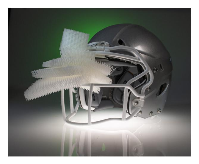
Researchers have developed microlattice impact attenuator pads that could make helmets better at protecting the wearer. Credit: HRL Laboratories, LLC
