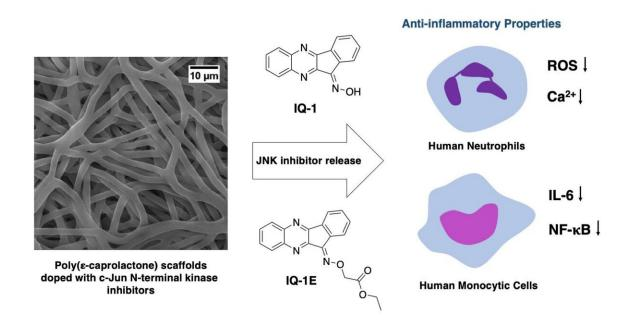
Mechanism of the developed materials: Composite scaffolds from polycaprolactone release the IQ-1 inhibitor and suppress the inflammatory response of immune cells. Credit: Tomsk Polytechnic University
