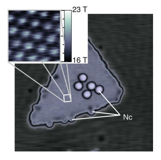
Topographic image of a small island of Cobalt on a Copper surface (size 25 Nanometer times 25 Nanometer). Nc mark the molecules used for functionalising the tip. The tiny square mark the area of a zoom-in which is shown enlarged in the top left corner and which shows the different magnetic interaction field from different Cobalt atoms in the layer.
