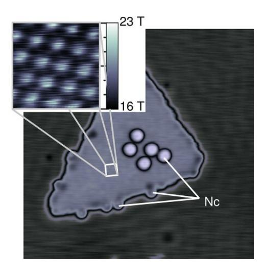
Topographic image of a small island of Cobalt on a Copper surface (size 25 Nanometer times 25 Nanometer). Nc mark the molecules used for functionalising the tip. The tiny square mark the area of a zoom-in which is shown enlarged in the top left corner and which shows the different magnetic interaction field from different Cobalt atoms in the layer. Credit: Forschungszentrum Jülich/Markus Ternes
