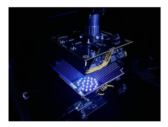
Duke Engineers have developed a new type of microscope that uses a bowl studded with LED lights of various colors and lighting schemes produced by machine learning. Credit: Roarke Horstmeyer, Duke University
