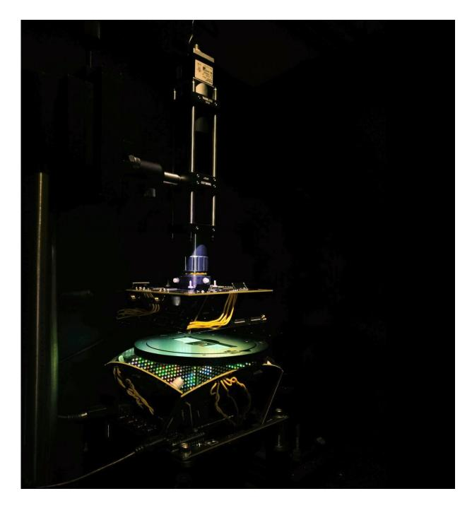
Duke Engineers have developed a new type of microscope that uses a bowl studded with LED lights of various colors and lighting schemes produced by machine learning. Credit: Roarke Horstmeyer, Duke University
