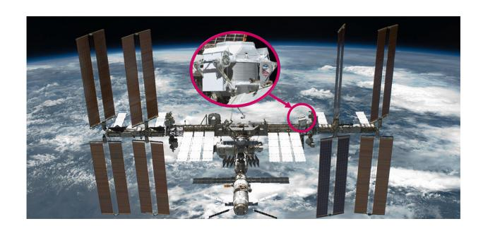
Particle physics detector, the AMS-02, is mounted on the upper Payload Attach Point on the S3 Truss of the International Space Station (ISS). Credit: AMS-02
