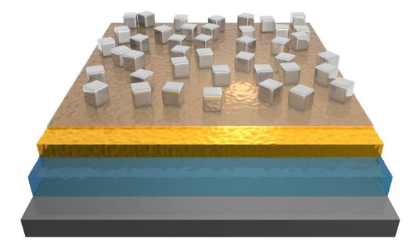
The new photodetectors allowing multispectral cameras with unprecedented frequency range are built from three layers. The size and spacing of silver nanocubes on a thin layer of gold dictates what frequency they absorb, causing them to heat up. A thin layer of a pyroelectric material called aluminum nitride then converts the heat to an electric signal, which is picked up and carried by a layer of silicon semiconductor on bottom. Credit: Jon Stewart, Duke University
