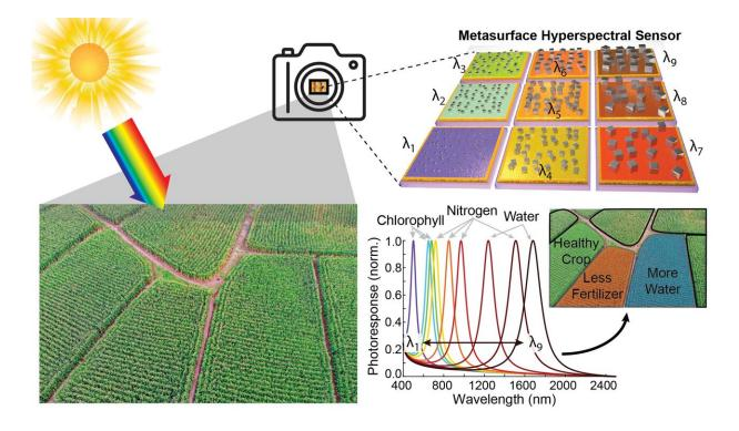
A new type of lightweight, inexpensive hyperspectral camera could enable precision agriculture. This graphic shows how different pixels can be tuned to specific frequencies of light that indicate the various needs of a crop field. Credit: Maiken Mikkelsen & Jon Stewart, Duke University
