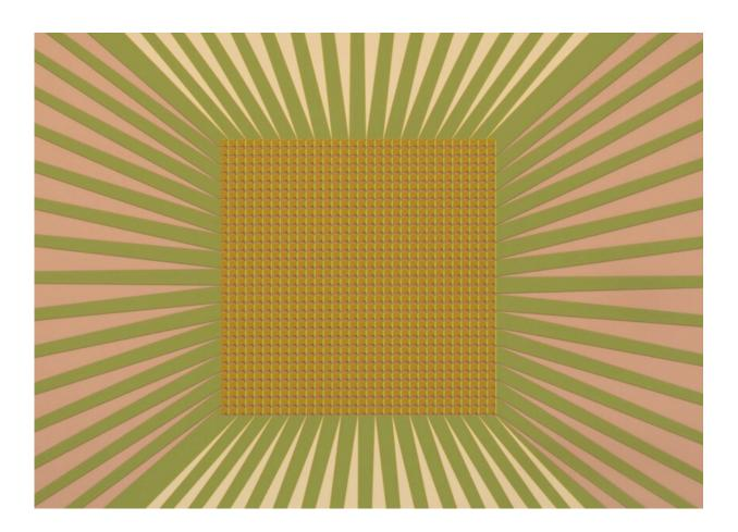
Micrograph of NIST's high-resolution camera made of 1,024 sensors that count single photons, or particles of light. The camera was designed for future space-based telescopes searching for chemical signs of life on other planets. The 32-by-32 sensor array is surrounded by pink and gold wires connecting to electronics that compile the data. Credit: V. Verma/NIST
