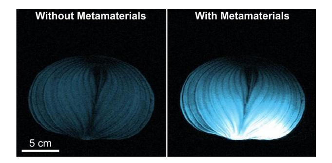
Two MRI images of an onion: the image on the right shows enhancement produced by an intelligent metamaterial developed by Xin Zhang and colleagues. Image courtesy of Zhang et al. Credit: Zhang et al.
