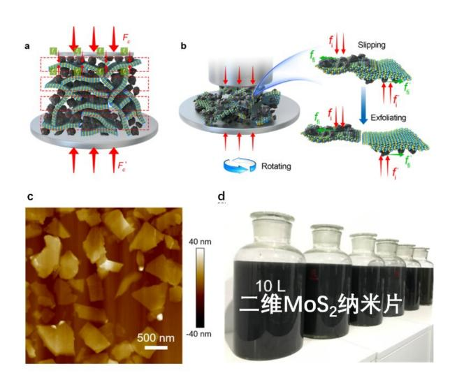
(a) Schematic of the decomposition of the macroscopic compressive forces Fc and Fc' into much smaller microscopic forces fi and fi? that were loaded onto the layer materials by force intermediates. (b) Exfoliation mechanism of layer
