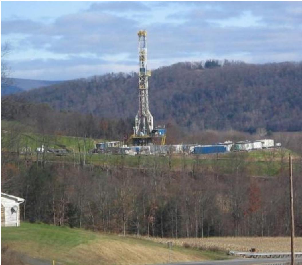
Derrick and platform of drilling gas wells in Marcellus Shale - Pennsylvania.
