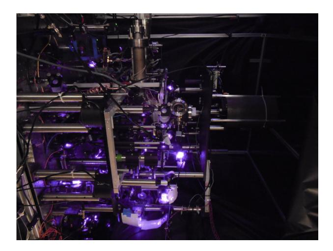
Laser light (purple) shines into our ultra-high vacuum chamber to laser-cool atoms to less than half a millionth of a degree above absolute zero. A pair of mirrors mounted inside the vacuum chamber enhance flashes of light which kick, suspend, and interfere the atoms. Credit: Victoria Xu
