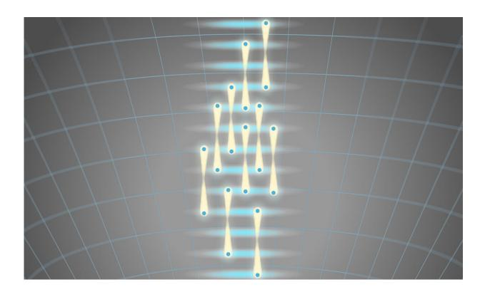
Atoms in a spatially-separated quantum superposition are suspended against Earth's gravity, using the standing wave formed by an optical cavity. Credit: Sarah Davis
