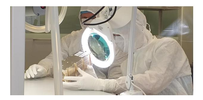
On behalf of the ESA, UCLouvain has developed antennas for the LaRa instrument that will go to Mars in 2020 to study the red planet's habitability. The originality of UCLouvain's concept: the antennas are produced from a single block of aluminium to achieve lightness (132g!), miniaturisation (hand-sized) and great resistance (particularly to day-night temperature variations of more than 200° C). Credit: UCLouvain
