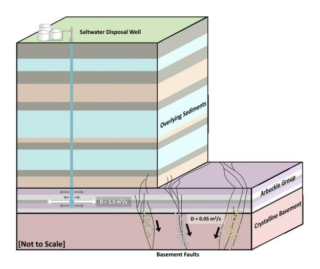
This simplified hydrology model shows the subsurface of Oklahoma. The Arbuckle Group is the area where most wastewater is injected. This layer allows fluid to move easily to distant areas. The added water causes stress as it travels and can cause earthquakes when it encounters pre-existing faults. Credit:
