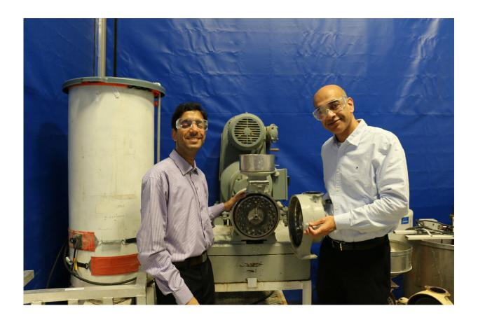
Chinmay Kurambhatti (left) and Vijay Singh show a pilot plant wet fractionation corn grinding mill located in the Integrated Bioprocessing Research Laboratory at the University of Illinois. Credit: Marianne Stein
