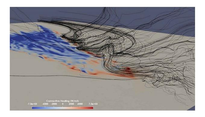
Stream traces of winds reaching the left flank and head of a simulated fire spreading up a steep slope. The blue region indicated the region that is actively burning and the residual fuel is being convectively cooled and the red region denotes locations where the fuel in front of the fire is being convectively heated. Credit: FIRETEC simulation generated by Alexandra Jonko (Los Alamos National Laboratory)
