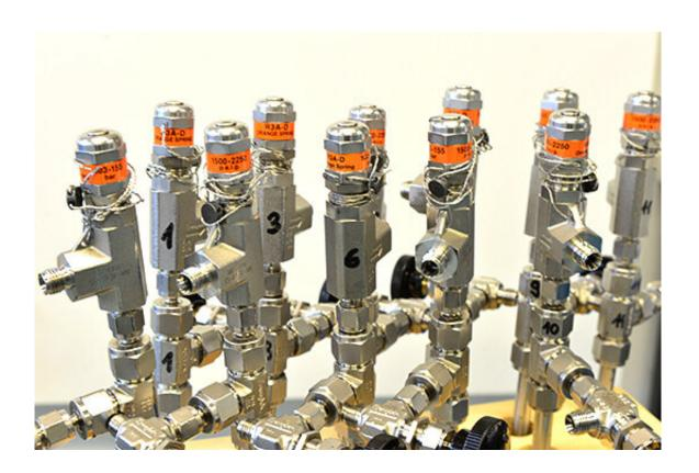
Reactors used for parallel screening of the effects of various pressures on formaldehyde synthesis. Credit: O. Trapp
