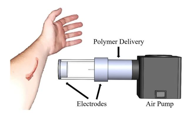
Illustration of the electrostatic and air driven device set up for direct deposition of a bandage onto a wound site. Credit: L.G. Huston and E.A. Kooistra-Manning, Montana Technological University
