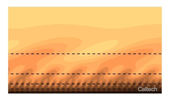
Modeled self-similar hierarchy in a turbulent boundary layer. Credit: California Institute of Technology
