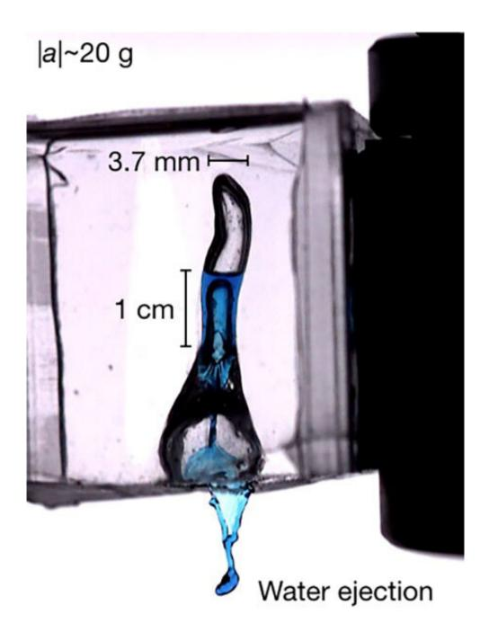
Various tube sizes and different accelerations were tried to determine what combination was necessary to remove water from a confined area. Credit: Anuj Baskota, Seungho Kim, and Sunghwan Jung
