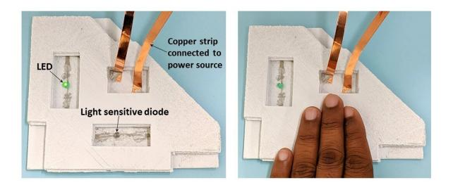
This is an example of simple light-sensing electronics with an LED (lightemitting diode), a light-sensitive diode (semiconductor) and power connected by a high-performance circuit inside polymer. The LED is on when exposed to light and off when light from the diode is blocked. Credit: Md Naim Jahangir
