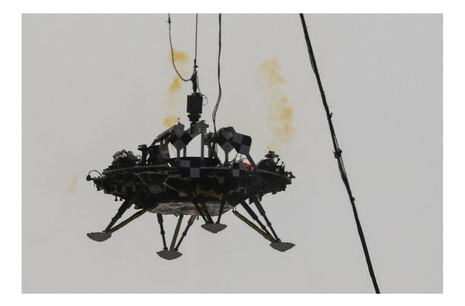
A lander is lifted during a test of hovering, obstacle avoidance and deceleration capabilities at a facility in Huailai in China's Hebei province, Thursday, Nov. 14, 2019. China has invited international observers to the test of its Mars lander as it pushes for inclusion in more global space projects. Thursday's test was conducted at a site outside Beijing simulating conditions on the Red Planet,
