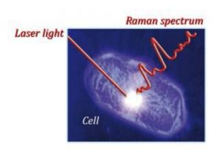
Raman microspectroscopy helps researchers observe cell chemistry by focusing a laser beam on a spot within a cell and then capturing light emitted after interactions with cellular molecules, which produces a molecular fingerprint (Raman spectrum). Credit: Stony Brook University
