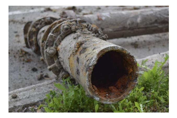
This June 19, 2019 photo shows corroded water pipes being replaced on Saint-Dominique Street in Montreal, Quebec, Canada. In Canada, where provinces—not the federal government—set water safety rules, the main source of lead in drinking water is antiquated pipes. At one government hearing, an expert estimated some 500,000 lead service lines are still delivering water to people in the country. (Mackenzie Lad/Institute for Investigative Journalism/Concordia University via AP)
