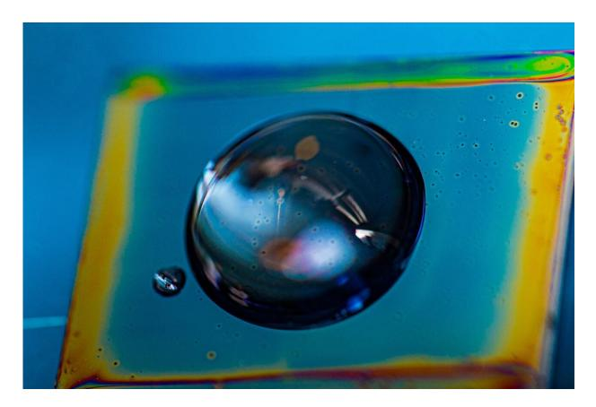
A hydrophobic coating of bottlebrush polymers created by Rice University engineers resists a drop of water. Microscopic bottlebrushes can be configured to give coatings specific properties for many applications. Credit: Jeff Fitlow/Rice University
