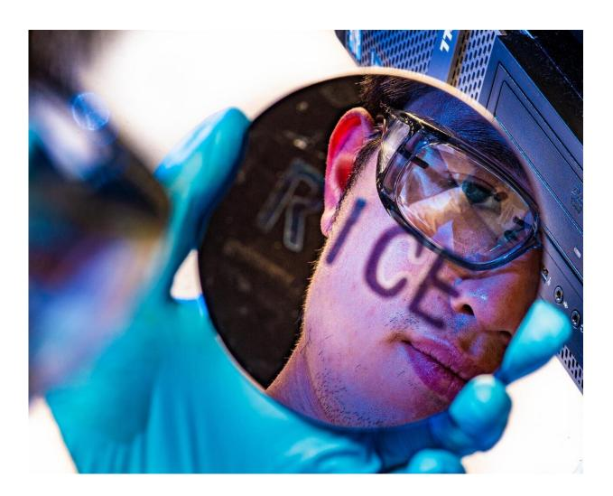
Rice University graduate student Hao Mei holds a plate with a pattern of bottlebrush polymers spelling "RICE." The microscopic polymers could give industry exquisite control over the properties of surface coatings. Credit: Jeff Fitlow/Rice University
