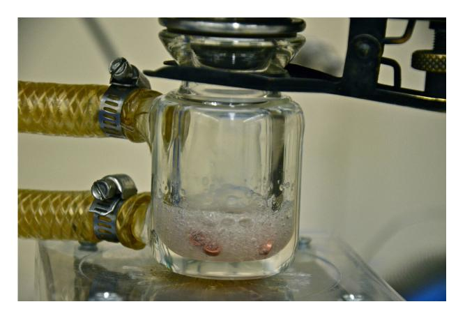
Sample reacting with phosphoric acid, releasing CO2 gas which will then be analyzed using mass spectrometry. Credit: Philip Staudigel
